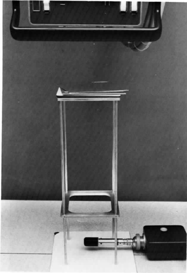
Figure 7.18a. HVL measurement setup for an overtable x-ray tube with a lead sheet under the dosimeter. The geometry for HVL measurements should be selected so that the aluminum filtration being added to make the measurement is placed halfway between the x-ray source and the ionization chamber. The x-ray beam must be collimated to an area just slightly larger than the ionization chamber.
